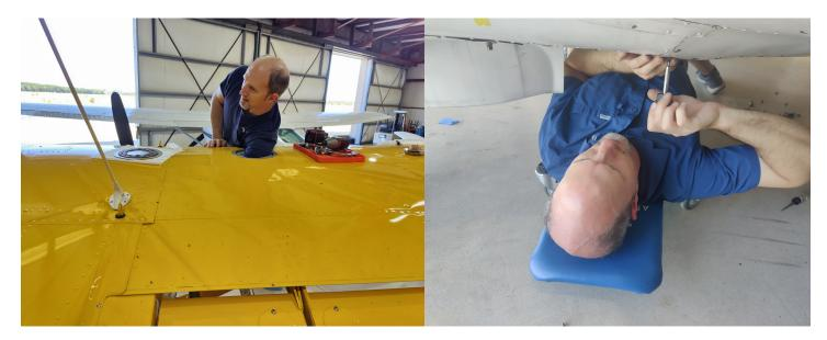
out. There are some things he has begun to master or already has mastered. Tying safety wire is one of them. It's used in correlation with cotter pins and other things to prevent fasteners from coming loose, and when the wire is applied, it needs to be tight, even, and secure. When Kyle is finished with it, it looks machine-done.
