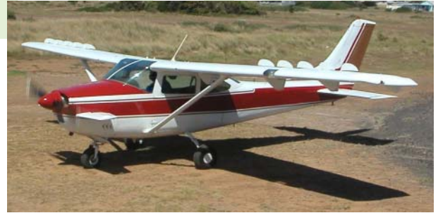
A Cessna 182 Wren - notice the canard on the nose and the Wren's teeth on the wings.
