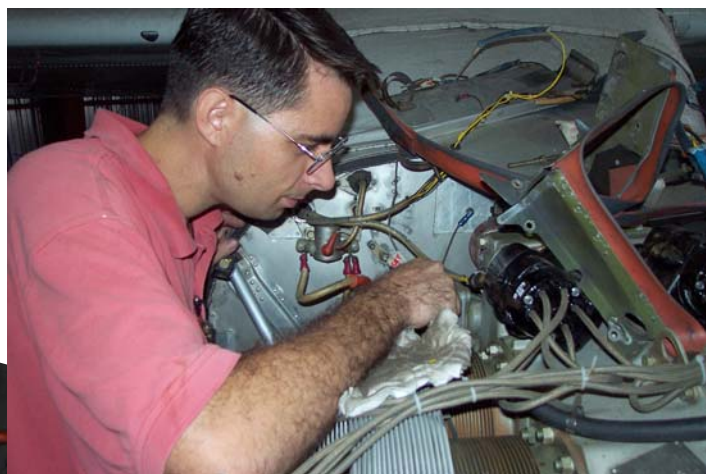
Left: Andy and Dwayne muscle the engine off of its mount with the help of a portable overhead chain hoist borrowed from our friends at the U.S. Embassy. Thank you! Below: Clifton inspects the new FM oil filter adapter installation.
