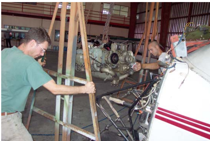
Left: Andy and Dwayne muscle the engine off of its mount with the help of a portable overhead chain hoist borrowed from our friends at the U.S. Embassy. Thank you! Below: Clifton inspects the new FM oil filter adapter installation.
